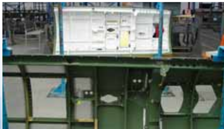
F/A-18 gun bay door production in AERO – E/F version (front), G version (back).
